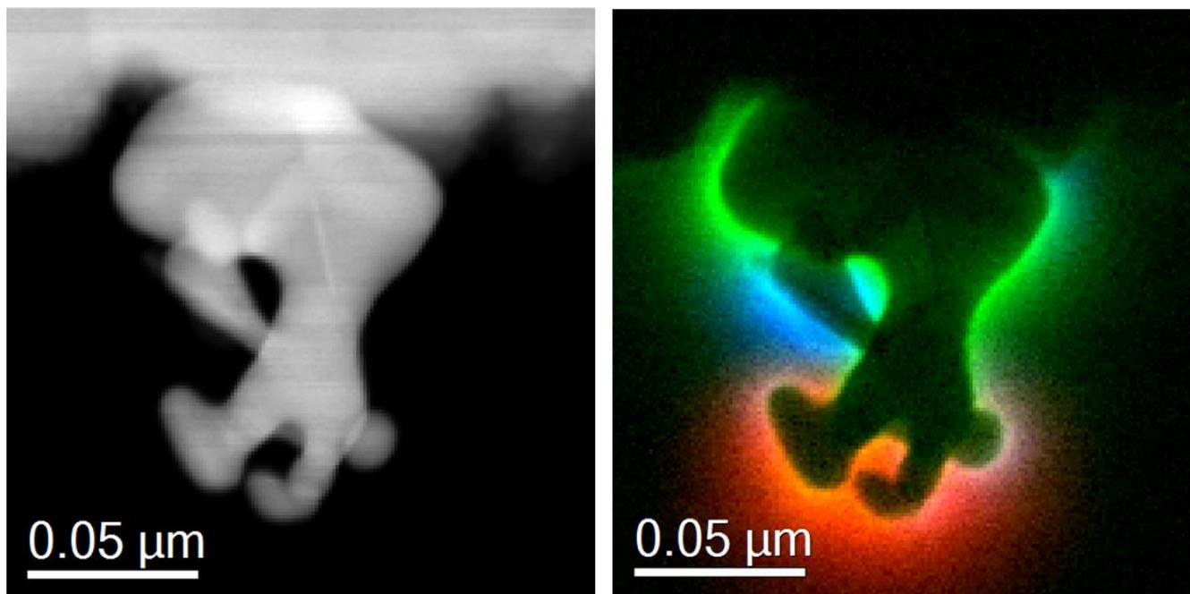
Figure 1. (left) HAADF image of a gold nanoparticle with irregular geometry. The top surface is a thin-film of SrTiO<sub>3</sub>. (right) RGB composite image by mixing the resultant weights of fitting three gaussians on an EELS Spectrum Image taken around the nanoparticle. The surface plasmon peaks are coloured in the following manner: Red: 1.46eV. Green: 2.4eV. Blue: 1.95eV.
